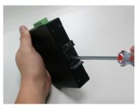
Step 1: screw the DIN-Rail on the Industrial Fast Ethernet Switch.
